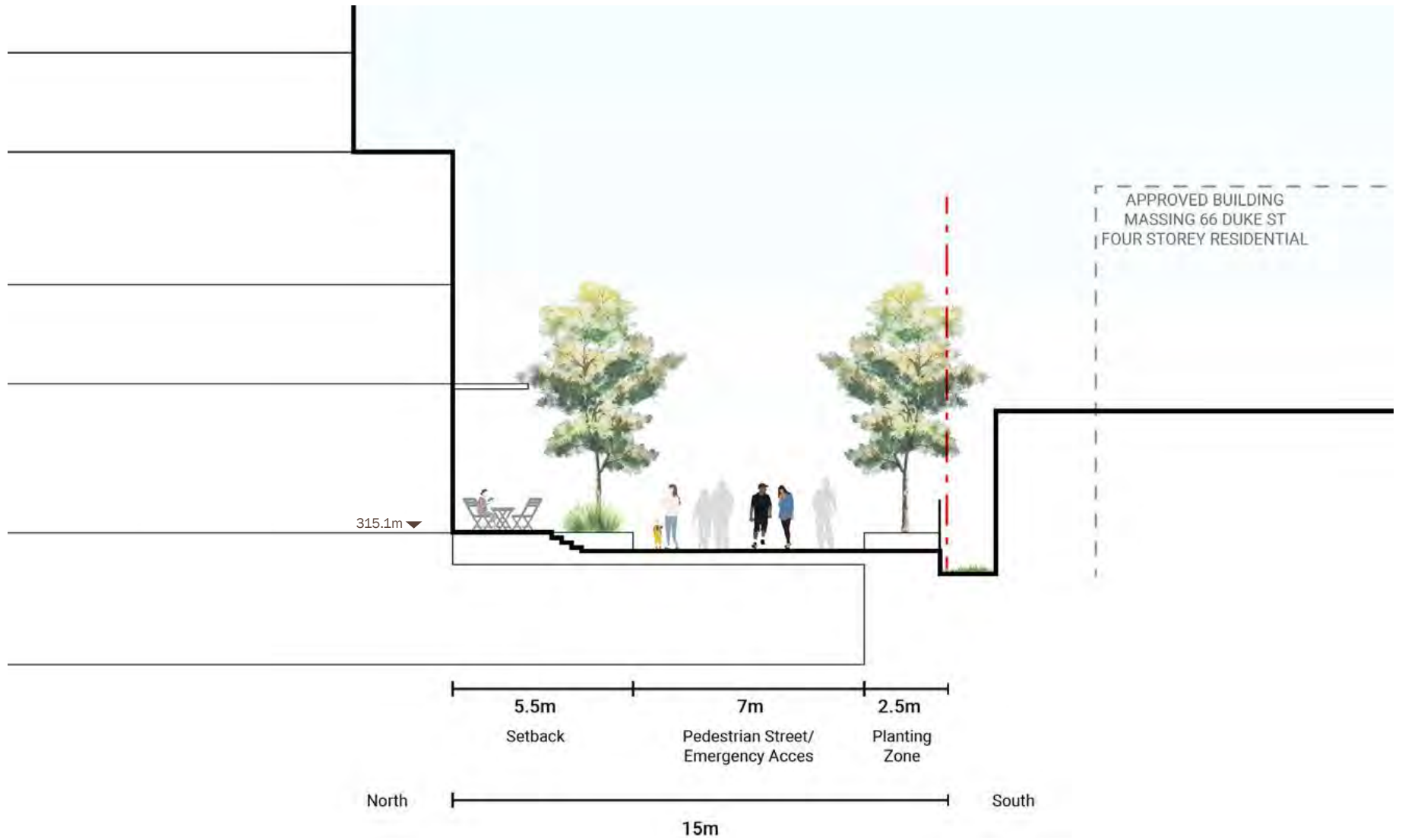
Figure 73. Duke Mews Cross-Section Looking East
