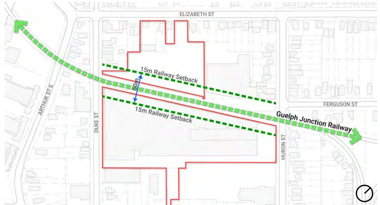
Figure 5. Rail corridor and setbacks
